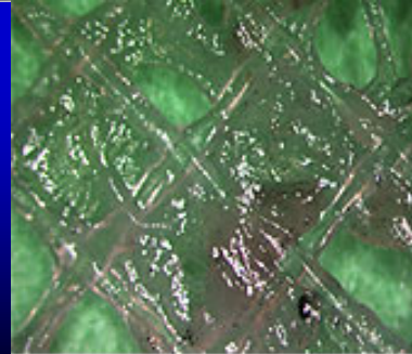
Fouled Feed Spacer
