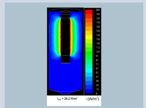
Fig. 3. Fluence rate distribution of low pressure UV lamp (wavelength A) in the UV batch reactor.
