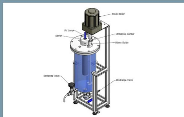
Fig. 1. UV batch reactor
