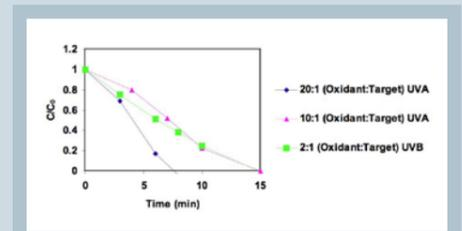
Fig. 4. Oxidation of IPA at  $100 \mu g l^{-1}$  with different oxidant dosages and different UV lamps (the concentration of IPA was expressed with  $\mu g$  TOC per liter).
