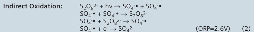
The  $\lambda_{max}$  of both persulfate and hydrogen peroxide is in the range of 194 to 200 nm. The molar extinction coefficient ( $\epsilon$ ) of persulfate is  $950 M^{-1} cm^{-1}$ , which is around four times higher than that of hydrogen peroxide ( $\epsilon = 265 M^{-1} cm^{-1}$ ). It indicates that persulfate might be a better oxidant for UV mediated AOP process.
