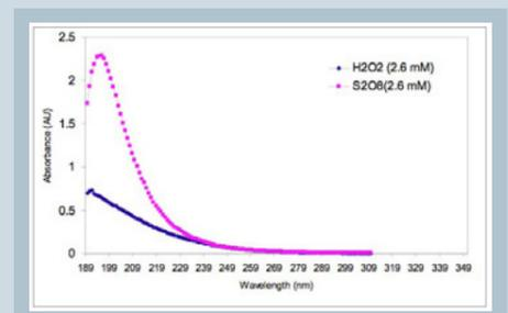
Fig. 2. Absorption spectra of persulfate and hydrogen peroxide.
