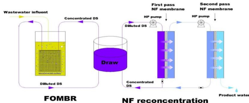
Figure 1. Schematic diagram of FO-MBR with NF process.
