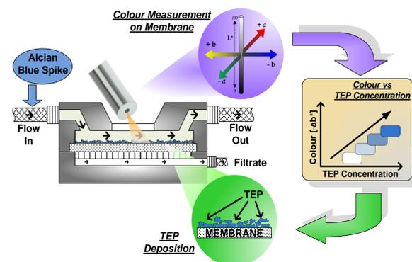
Figure 1: Schematic diagram of TEP sensor
