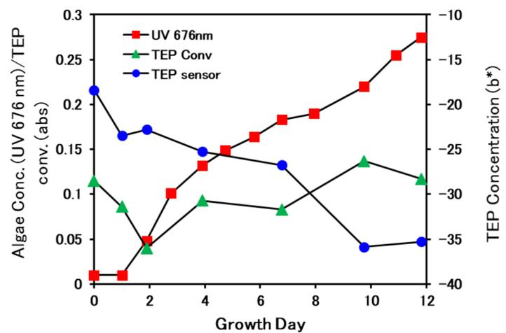
Figure 4: Changes in cell density, conventional TEP (TEP>0.1µm) and TEP sensor (TEP>30kDa) measurements during the incubation period of batch culture of *Thalassiorra Pseudonana*. Note the TEP sensor was performed at lower flux of 90L/m<sup>2</sup>.h, filtration duration of 2 hours.
