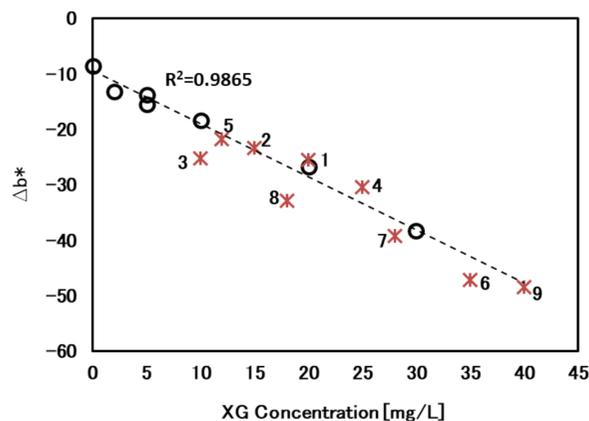
Figure 3: Calibration between  $\Delta b^*$  and XG concentration (o). The red stars (\*) are the values obtained after each cycle of regeneration. The number beside the star indicates the sequence of the test. Conditions: Flux = 180L/m<sup>2</sup>.h; crossflow velocity = 0.15m/s, filtration duration 30 minutes
