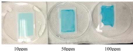
Figure 2: Different concentrations of XG fouled on 30kDa membrane surface, stained with AB.
