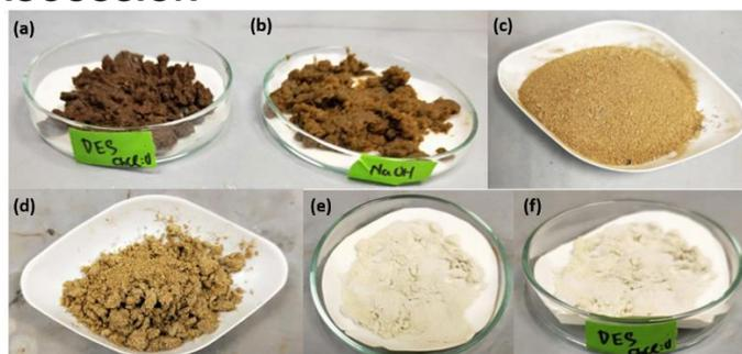
**Figure 3:** Pictures of (a) Wet DES-treated rice husk, (b) Wet alkaline-treated rice husk, (c) Dried ground DES-treated rice husk, (d) Dried ground alkaline-treated rice husk, (e) Dried bleached alkaline-treated cellulose fiber and (f) Dried bleached DES-treated cellulose fiber
