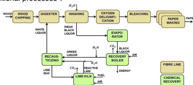
**Figure 1:** Process flow of conventional Kraft pulping and paper milling
