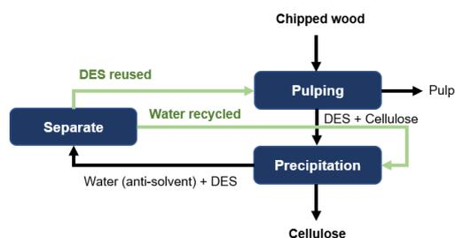
**Figure 2:** Proposed process of pulping incorporated with DES
