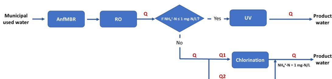
**Figure 1** Illustration of the integrated AnfMBR-RO-Chlorination process.
