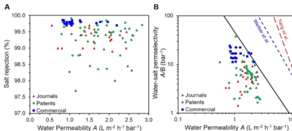
**Fig. 1.** Performance data of all the SWRO membranes summarized in this work, including journal papers, commercial and patents (sample size: 105). Raw plot of **(A)** water permeability and NaCl rejection and log-log plot of **(B)** water permeability and water-salt permselectivity ratio  $A/B$ . The new SWRO upper-bound relationship (black solid line) is proposed based on the empirical data summarized.
