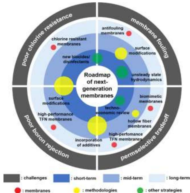
**Fig. 2.** Technology roadmap of the SWRO membrane fabrication, showing different short- and long-term strategies. The size of the circle represents the impacts they are likely to make towards next-generation SWRO membranes.
