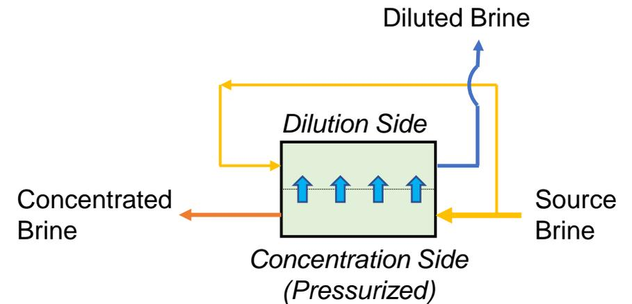
Schematic Diagram of a Single Stage Membrane BC System
