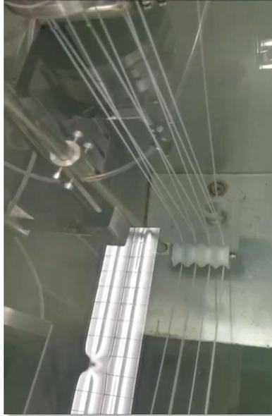
8-Channel Hollow-Fiber Spinning Line
