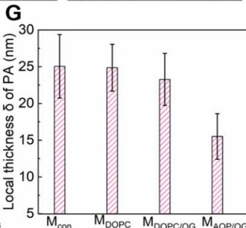
The constituents in the proteoliposome could facilitate the formation of a PA layer with enlarged protuberances and thinner crumples, resulting in a 79% increase in effective surface area.
