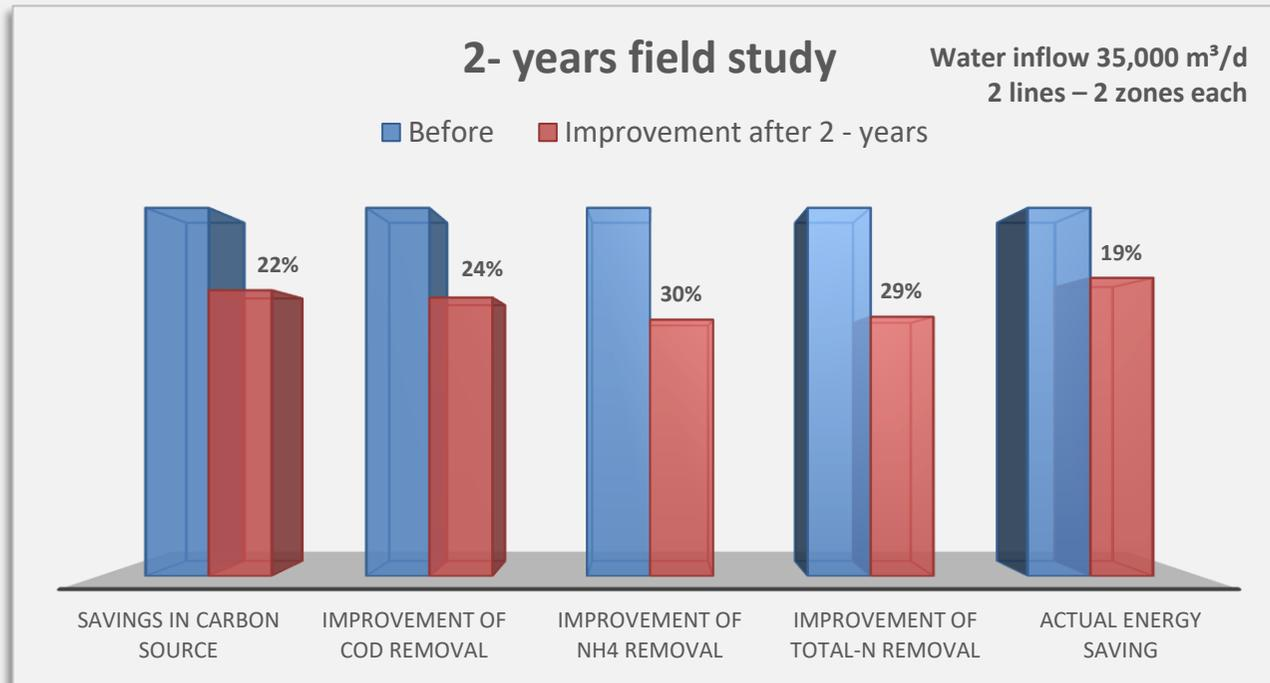
**Results:** Reduction of total nitrogen in the effluent with **19%** less energy consumption plus **22%** savings in chemicals
